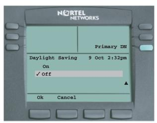
3. Press **Ok** to turn on Daylight Savings or press **Cancel** to return to the Time menu. Use the down navigation button to access the following screen in which you can turn off Daylight Savings.
